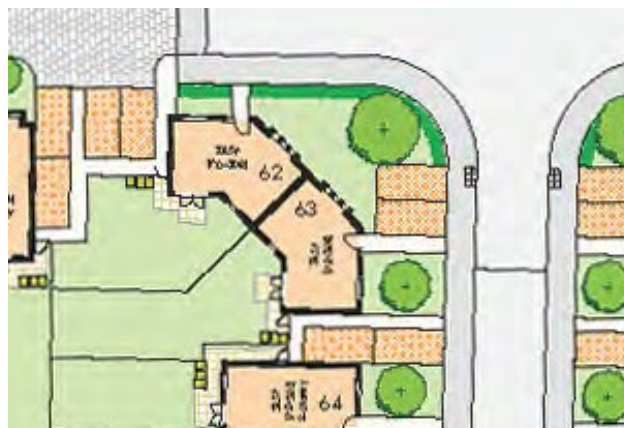
Bin storage areas shown on a layout drawing to demonstrate that these servicing requirements have been addressed (Drawing courtesy of Walker Troup Architects).
