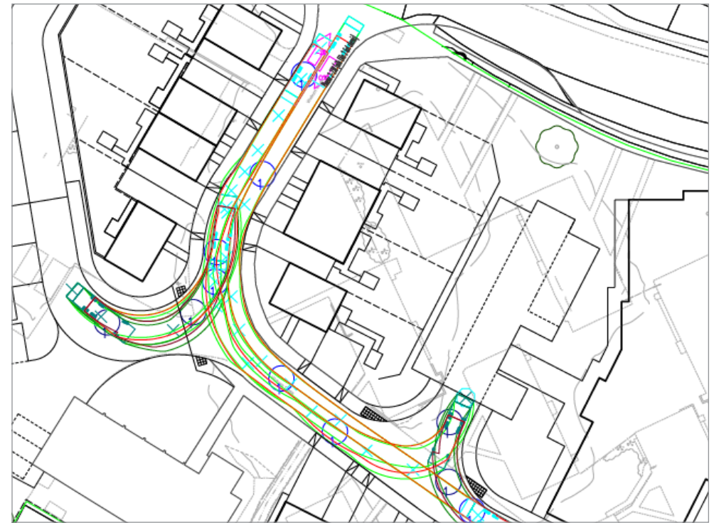
Above: Vehicle tracking demonstrating access and turning within the site is capable by a large refuse collection vehicle at Woburn Close, Blackwell. (Drawing courtesy of William Saunders. October 2023)
